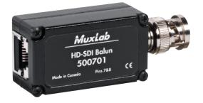
The HD-SDI Balun allows one HD-SDI signal to be transmitted up to 150 ft (45m) via Cat5e cable at HD resolution in a point-to-point configuration. The HD-SDI Balun supports transmission of up to 2.97/3.0 Gbps uncompressed, un-encrypted digital video (optionally including embedded Audio and/or Time Code) within television facilities and between professional video equipment.
