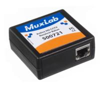
The Active HD CCTV Receiver Balun (500721) provides extended distance between an HD-SDI CCTV camera and an HD-SDI DVR via Cat5e/6 cable. The product supports up to 150 ft (45m) via Cat5e cable at HD (720p, 1080i) resolution when used in conjunction with MuxLab's HD CCTV Pass-Thru Balun (500720). Furthermore, the 500721 allows remote power and 2-wire PTZ control to be combined with HD- SDI video over the same Cat5e/6 for optimized cabling.
