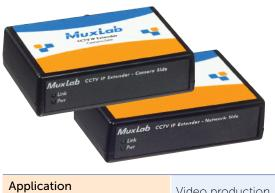
The CCTV IP Extender Kit (500110) allows any CCTV IP camera to be connected over extended distance via Cat5e or coax cable. The 500110 supports up to two IP cameras up to 650 ft (200m) at 100 Mbps and up to 1 mile (1.6km) at 25Mbps.
