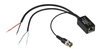
The HD CCTV Pass-Thru Balun with Cable Leads (500720-CL) allows one HD CCTV (HD- SDI) video channel plus remote power and PTZ control to be transmitted between the HD CCTV camera and the DVR via Cat5e/6 cable in the HD CCTV environment. The 500720-CL is used in conjunction with either another 500720-CL or in conjunction with the 500720-CL or 500721.
