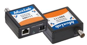
The CCTV IP PoE Extender (500111) allows one IP camera (14 Watts) to be connected up to 1600 ft (500 m) via a single 75-ohm coax cable in a point-to-point configuration. The product works in pairs and the power consumption is low enough so that it does not load the PoE source or switch. The maximum distance depends on the grade of coax cable and the power consumption of the camera.
