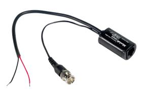
The CCTV Power-Thru Balun allows video and remote power to be transmitted via one 4-pair Cat5e/6 cable, thus eliminating the need to install multiple cables for more efficient cabling in the CCTV security and surveillance environment. The Power-Thru Balun may be used in pairs or in conjunction with standard twisted pair crossconnect devices and other MuxLab CCTV baluns such as the 500000, 500009, 500023 and 500015.
