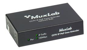
The LongReach CCTV IP PoE Extender Kit (500112) allows one CCTV PoE IP camera (up to 15.4 Watts) to be connected up to 980 ft (300 m) via a single 75-ohm coax cable in a point-to-point configuration to a PoE LAN switch. If the LAN switch is not PoE, then the 48VDC Power Supply (500113) is required in order to power the PoE camera and the 500112. The maximum distance depends on the grade of coax cable and the power consumption of the camera.
