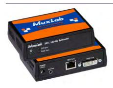
The DVI/Audio Extender Kit (500390) allows one DVI channel and one line level 2CH audio signal to be transmitted up to 230ft (70m) at all resolutions up to 1080p via one (1) Cat5e/6 cable in a point-to-point configuration.
