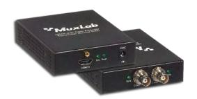
The HDMI over Coax Extender Kit (500465) allows an HDMI source to be connected to an HDMI receiver up to 250ft (76m) at 1080p resolution via one (1) coax cable in a point-to-point configuration. Furthermore, the product may be cascaded via the HDMI over Coax Receiver (500465-RX) in order to support multi-display applications.
