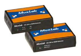
The 3G-SDI to HDMI Extender Kit (500715) converts 3G-SDI to HDMI and then transmits it up to 330ft (100m) via Cat5e/6 cable at all resolutions in a point-to-point configuration. The 3G-SDI to HDMI Extender supports transmission of up to 2.97/3.0Gbps uncompressed, un-encrypted digital video (optionally including embedded Audio and/or Time Code) within television facilities and between professional video equipment.
