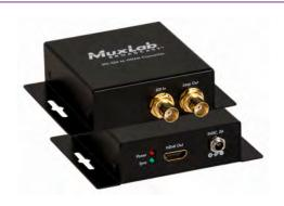
The 3G-SDI to HDMI Converter allows SDI equipment to be connected to an HDMI Display. The unit converts the SDI signal to HDMI, supporting resolutions of 480i (SD-SDI), 720p/1080i (HD-SDI) and 1080p (3G-SDI). The 3G-SDI to HDMI Converter provides a low jitter and re-clocked outputs allowing for unit daisy chain.
