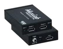
The DisplayPort 1.2a 1x2 Splitter, SST allows you to duplicate identical DisplayPort 1.2a content from one DisplayPort connector to two monitors. The splitter supports video resolutions up to 4K and PCM Audio up to 7.1-Channel and up to 192 kHz sampling rate, supporting a Single Stream Transport (SST).
